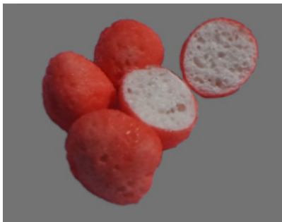
Figure 1: Wax coated Poraver particle
