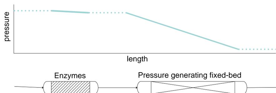
Fig 2: Currently planned reactor setup. First fixed bed contains immobilized enzymes
