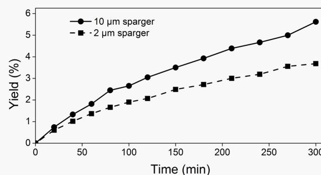
Fig. 4: Conversion of resorcinol to 2,6-DHBA by decarboxylase during  $\text{CO}_2$  aeration. The reactions were performed at 100 mL  $\text{CO}_2/\text{min}$  with different sparger pore sizes and otherwise identical reaction conditions.
