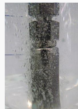
Fig. 3: Bubble aeration with 10  $\mu\text{m}$  sparger
