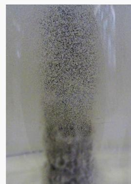
Fig. 2: Bubble aeration with 2  $\mu\text{m}$  sparger
